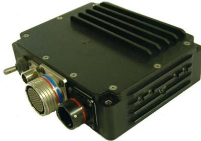
The 40A voltage regulator and powerbox is designed to be used in combination with a permanent magnet alternator. The variable three-phase input voltage from the alternator is full-wave rectified and smoothed to provide a DC low-impedance source to the regulator. The output voltage can be set to the customer's requirements.
